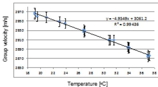
**Figure 2.** The group velocity results from the three repetitions of the measurement procedure together. Vertical bars indicate the expanded uncertainties.
