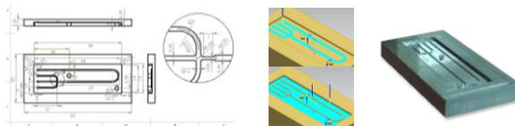
**Figure 1.** Manufacturing process realization: (a) technical drawing of a mould with micro features; (b) CAM tool path generation of operations; (c) machined exemplary mould.
