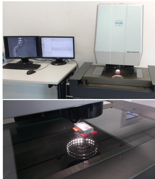
**Figure 2.** Multisensor CMM (top) selected for checking the dimensional content of microfluidic moulds (bottom).
