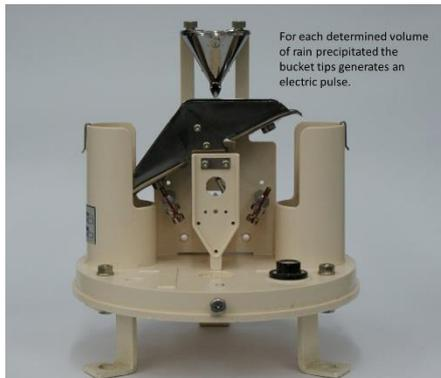
**Figure 1** - The TBRG and its measuring principle
