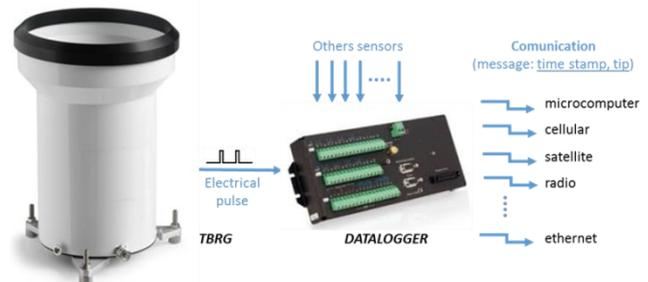
**Figure 2** - Schematics of a weather station with rainfall record.
