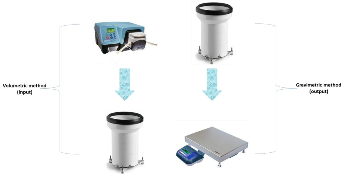
**Figure 3** - Calibration methods for a TBRG.
