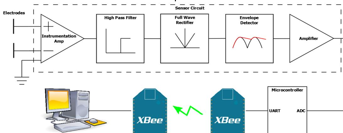
Figure 1. Schematics of the system
