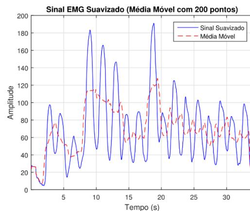
Figure 3. Smoothed EMG signal (solid blue curve) and variable amplitude threshold (dashed orange curve).
