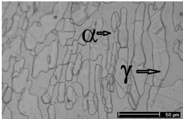
Fig. 2. The microstructure of the stainless steel as-received, where  $\alpha$  is the ferrite phase and  $\gamma$  the austenite one.
