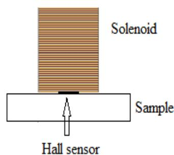
Fig. 1. Position of the sensor.
