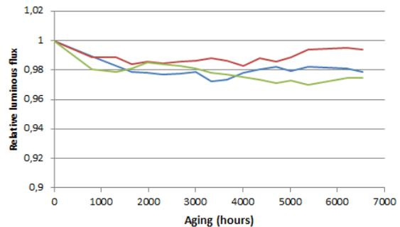
Figure 2: Relative luminous flux of 3 COBs used in the tests
