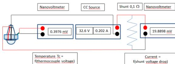
Figure 6 – Instruments and connections to the DC supply, and measurements of the current and Tc temperature
