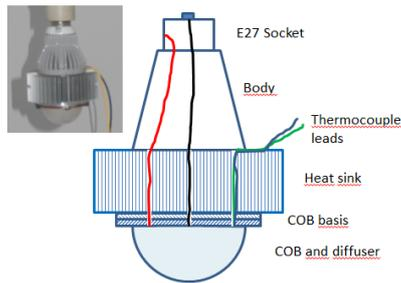
Figure 4 – Image and schematic drawing of the prototype
