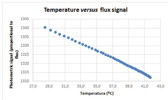
Figure 5 – Luminous flux as a function of Tc temperature during an interval of 60 minutes (supplied current 0.202 A).
