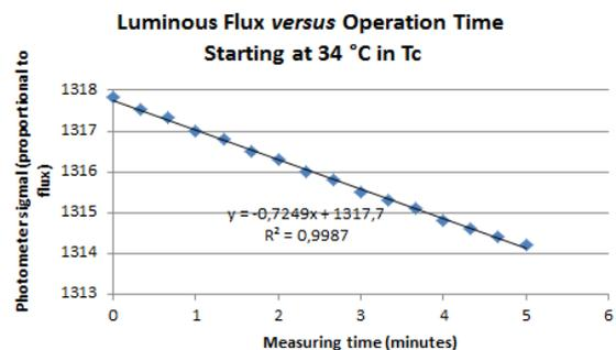
Figure 7 – 16 readings of luminous flux made during a 5 minutes period
