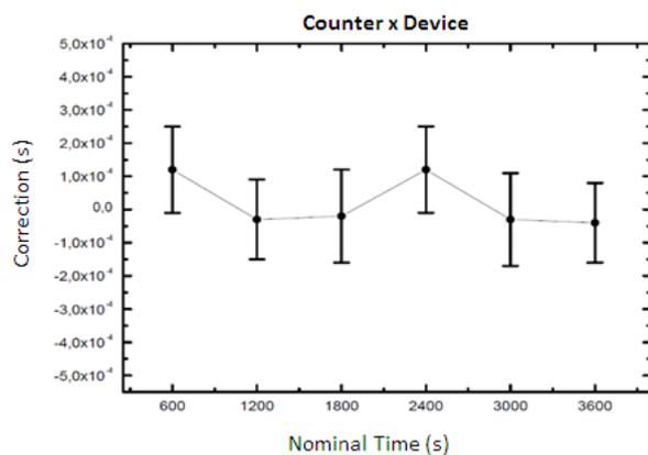
**Figure 2.** Correction chart x time referring to the time difference between the counter and the device.
