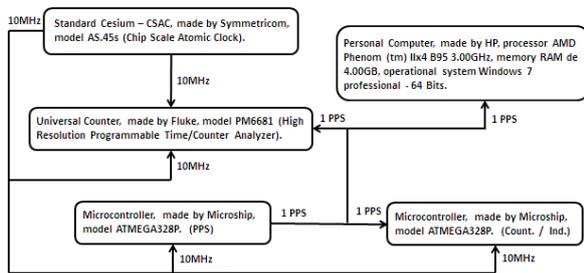
**Figure 1.** Connection diagram from Standard Cesium at Microcontroller device and to computer timer.
