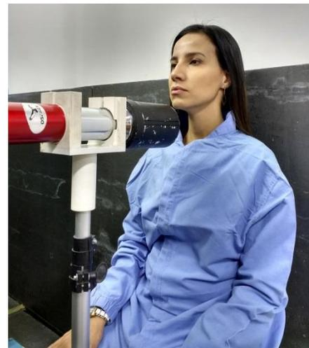
**Figure 2. *In Vivo* measurement of  $^{131}\text{I}$  in the thyroid, using a Pb-collimated NaI(Tl)3x3 installed on a tripod in Lab 1**
