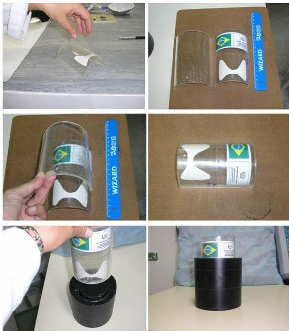
**Figure 1. Neck-thyroid phantom developed at IRD**
