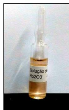
Figure 1. Candidate CRM of  $\text{Ho}_2\text{O}_3$
