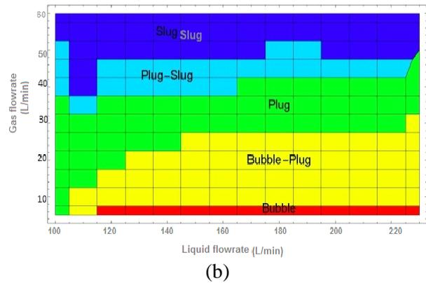
Figure 4 Maps of two-phase flow patterns for pipes of diameters 25 (a) and 50 mm (b).
