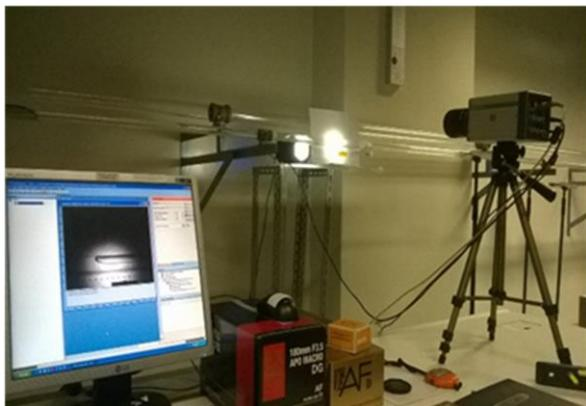
Figure 2 Shadow Sizer system at the visualization section.
