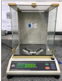
Figure 1. Semi-Analytical Balance - GEHAKA BG400
