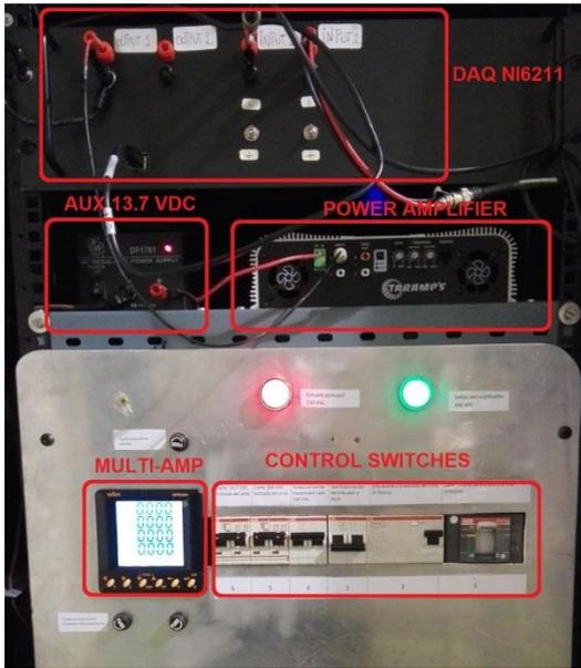
Fig 3. Power voltage source panel.
