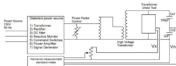
Fig 5. General diagram of the measurement system.
