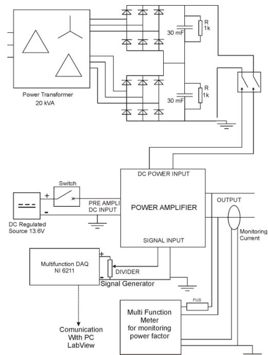
Fig 2. Power voltage source block diagram.
