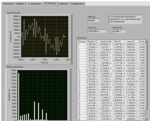
Fig 7. Primary waveform screen.
