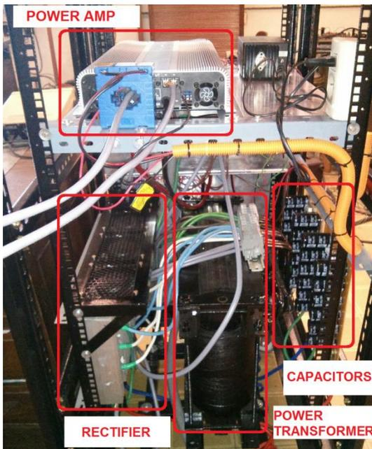
Fig 4. Internal view of the power voltage source.
