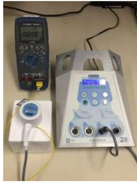
**Figure 1.** Experimental arrangement used for determining ultrasonic power with the calorimeter.
