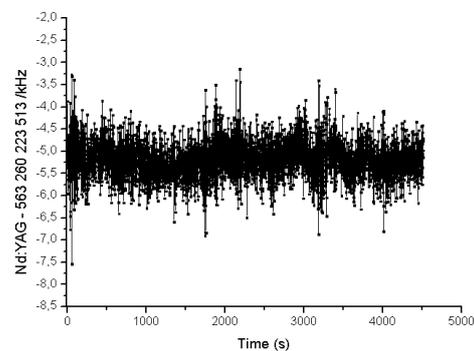
Figure 4 - Time record of measurements of the Nd:YAG frequency compared to the  $MeP$  value.
