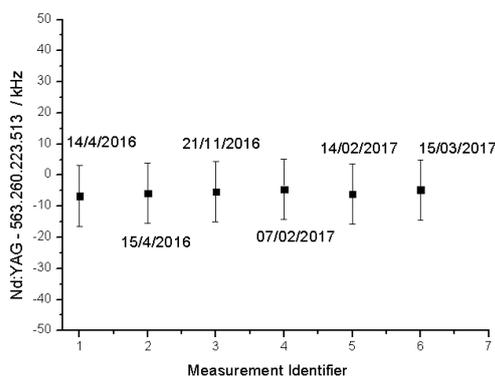
Figure 6 - Measurements of the Nd:YAG frequency compared to the MeP value.
