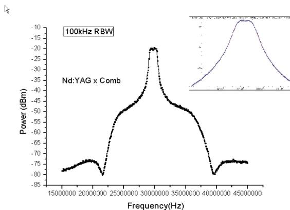
Figure 3 - Nd:YAG and comb beat note after filtering (filter center: 30MHz, 3 dB bandwidth 25 MHz-35 MHz) and amplification.
