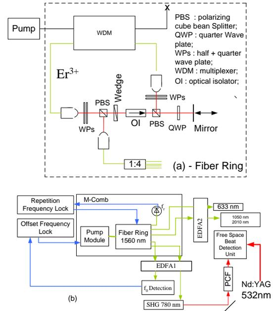
Figure 1 - FC 1500 setup. The green lines represent the fiber connection, blue lines the electrical/RF connection and the red lines the free space laser radiation.
