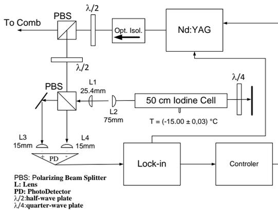
Figure 2 - Schematic diagram of the  $I_2$  stabilized Nd:YAG.
