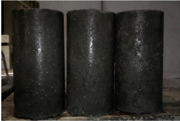
**Figure 2.** Cylindrical test specimens 10 centimeters in diameter and 20 centimeters in height.
