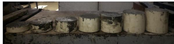
**Figure 1.** Cylindrical test specimens 2 to 8 centimeters in height and 10 centimeters in diameter.
