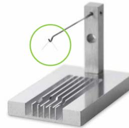
Figure 4. Wire weight with the nominal value of 0.05 mg loaded on the hook of an a10XL weight carrier.
