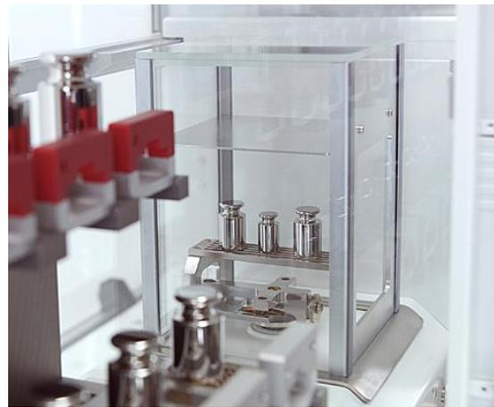
Figure 8. Three weights loaded symmetrically on the weighing pan of the a107 robotic comparator for dissemination.
