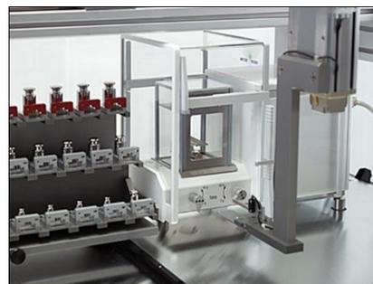
Figure 3. Switching dial weights of a107 comparator.
