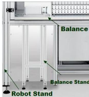
Figure 5. Separate stand of ultra-microbalance.
