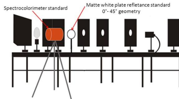
**Figure 1.** System for measuring standard lamps in correlated color temperature together with the Inmetro' photometry system.
