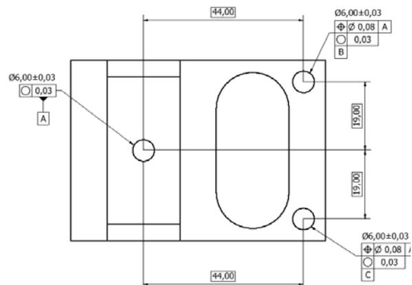
Figure 2 – Technical drawing of the tolerated elements
