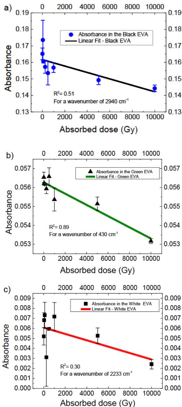
**Figura 4.** Integral area *versus* absorbed dose, using the FTIR technique and wavelengths from 190 nm up to 400 nm. (a) Black sample for a wavenumber of  $2940\text{ cm}^{-1}$ ; (b) Green sample for a wavenumber of  $430\text{ cm}^{-1}$ , (c) White sample for a wavenumber of  $2233\text{ cm}^{-1}$ .
