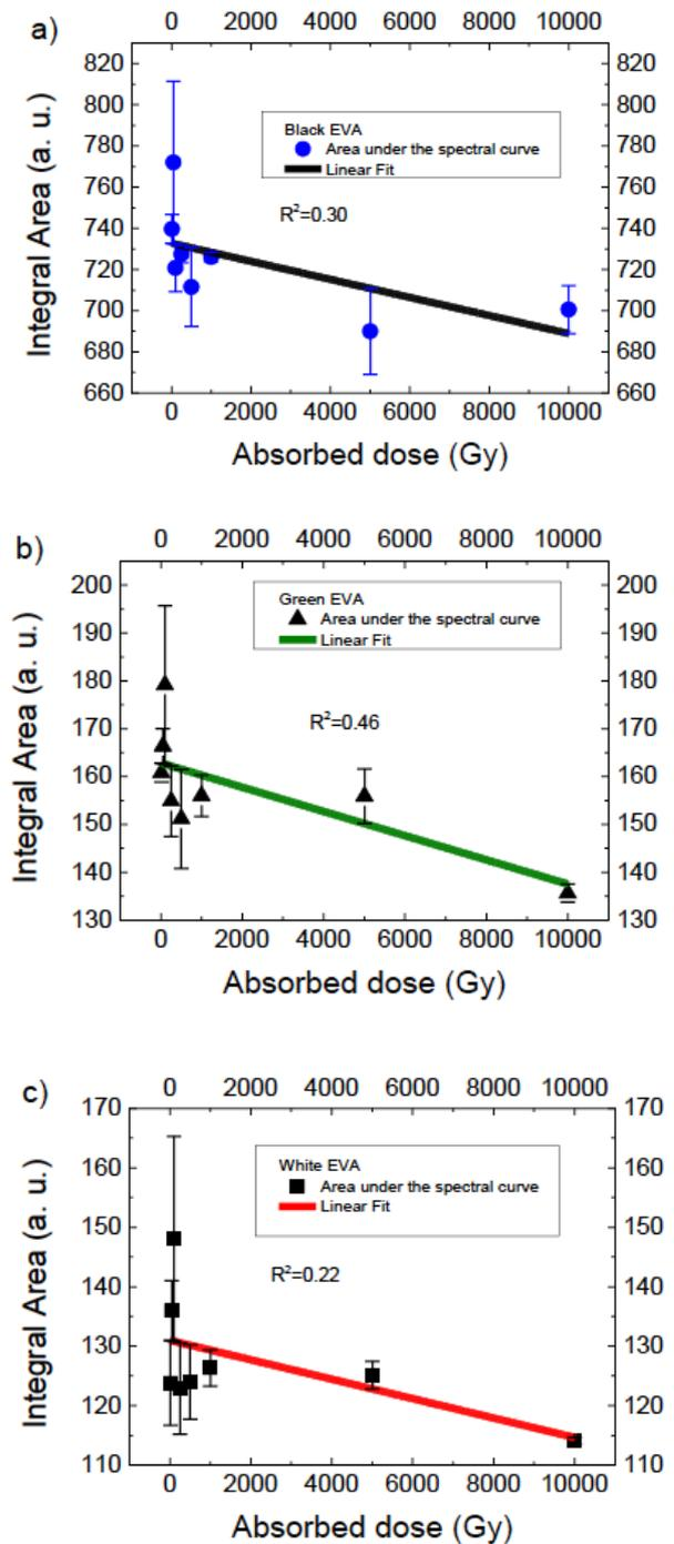
**Figure 3.** Integral area *versus* absorbed dose, using the FTIR technique and irradiation from 10 Gy up to 10 kGy of absorbed doses. (a) Black; (b) Green; and (c) White samples.
