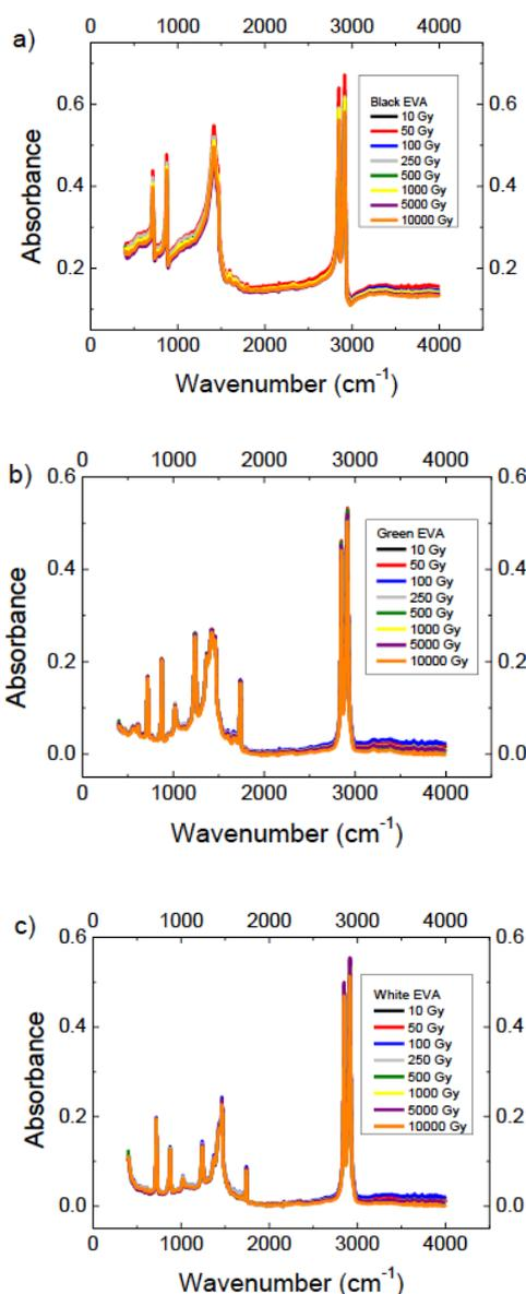
**Figure 1.** FTIR spectrum for EVA samples irradiated with absorbed doses of 10 Gy to 10 kGy. (a) Black; (b) Green; and (c) White. The average of 3 samples was evaluated for each
