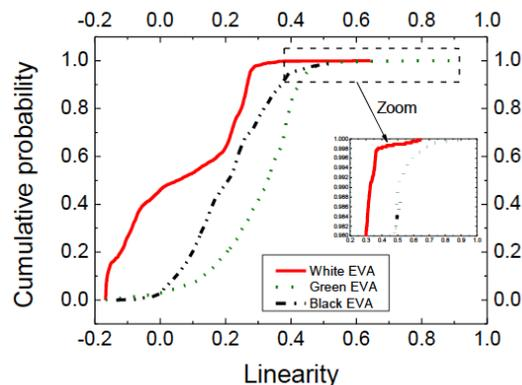
**Figura 5.** Cumulative probability *versus* linearity, for white, green and black EVA samples for wavenumber shown 400 up to  $4000\text{ cm}^{-1}$ .
