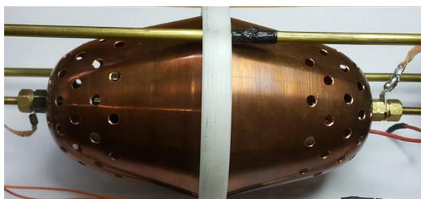
Fig. 1. Electrostatic shield made by two metallic cones.
