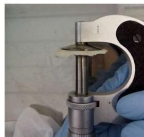
**Figure 1.** Measurement of porcine skin sample thickness by micrometer.
