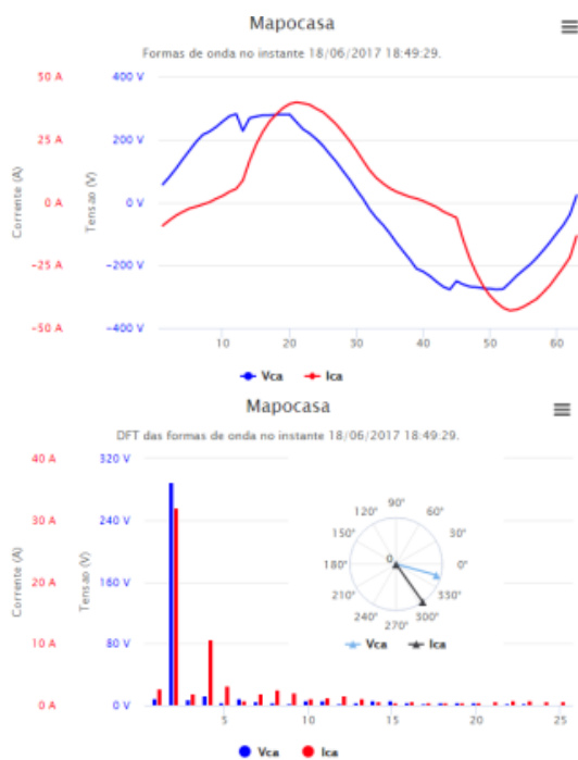
(d) No PV generation, TRIAC switched heater, 1 air conditioning unit, 1 refrigerator, some lamps
