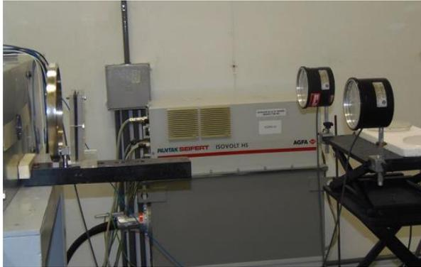
**Figure 1** – LCD/CDTN x-ray calibration set-up for calibrating the 2575NE chamber against the LNMRI/IRD national standard.
