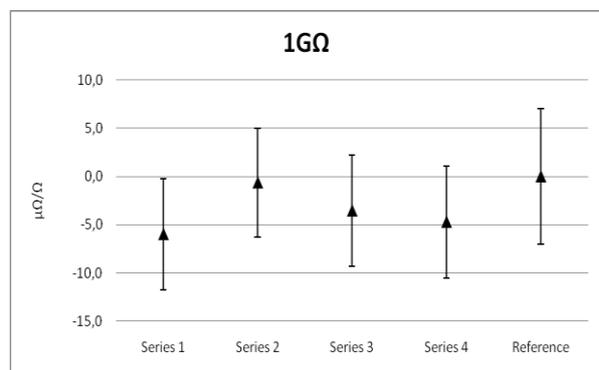
Figure 5 - Measured values for the 1 GΩ resistor.
