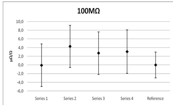
Figure 4 - Measured values for the 100 MΩ resistor.
