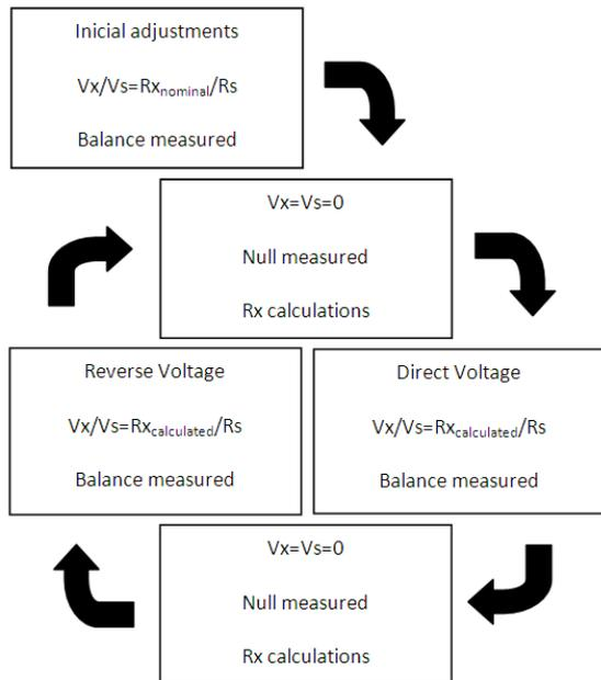
Figure 2 - Simplified diagram of the balancing algorithm.
