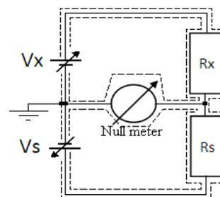
Figure 1 - Simplified schematic diagram of the modified Wheatstone bridge with voltage sources  $V_x$  and  $V_s$ , null-detector, reference resistor  $R_s$  and unknown resistor  $R_x$ . Dashed lines indicate the shielding of cables and resistors.
