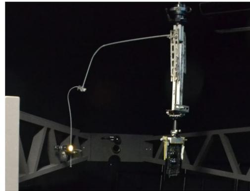
*Figure 4 – Mounting diagram for measurements of the retroreflective characteristics. On the right side we have the surface for placement of the body of evidence and, on the left, the light source. (IPT, 2017).*
