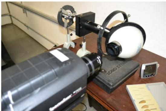
*Figure 3-Measuring assembly diagram of the CCT of the light source. In the right corner the filters used for adjusting the CCT of the light source (flashlight)( IPT, 2017).*
