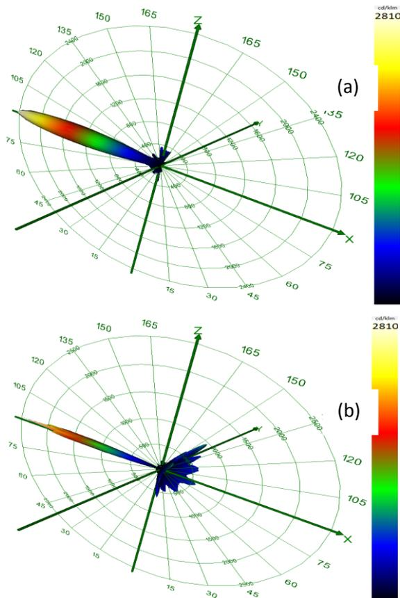
Figure 5 – Distribution of luminous intensity obtained from (a) projector and (b) Retroreflective material (IPT, 2017).
