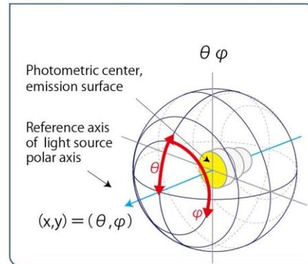
Figure 2 – Graphical representation of the Goniophotometers type C, in the center is positioned the luminous body to be measured, and on the axes in red are represented the axis of the sensor's offset. The illuminator was held fixed and aligned to the normal surface of the reflector. (Located in : <https://www.otsukael.jp/upload/files/GP%281%29.jp> g Accessed on: ago 2017).
