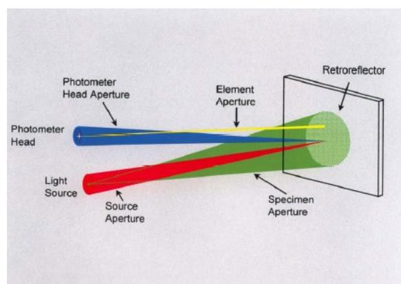
Figure 1 – Illustration of aperture angles for Retroreflection (CIE 54.2, 2001).
