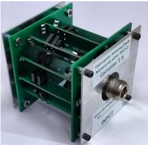
**Fig. 2.** 1 A shunt assembled at Inmetro.
