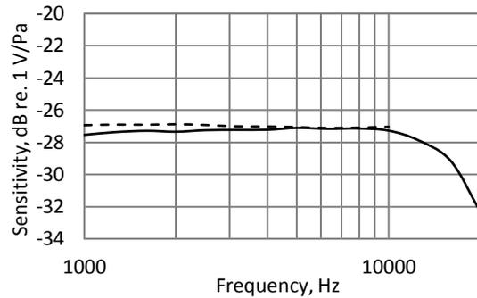
**Figure 6.** Diffuse-field sensitivities for one of the three half-inch microphones measured. — sensitivity obtained by the proposed procedure and - - sensitivity obtained by the comparison method.
