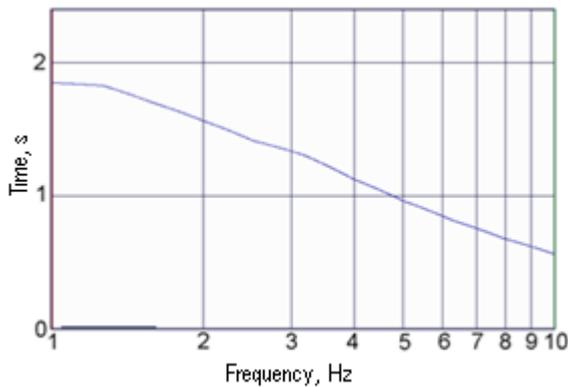
**Figure 5.** Chamber's reverberation time.
