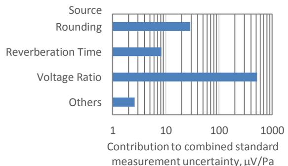
**Figure 7.** Contribution to combined standard measurement uncertainty at 3.15 kHz.
