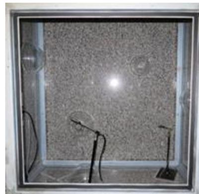
**Figure 3.** Reverberation chamber with boundary diffusers and microphones inside it.
