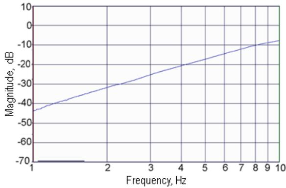
**Figure 4.** Electrical transfer impedance between a pair of microphones. Average between measurements performed at twenty-four different positions.
