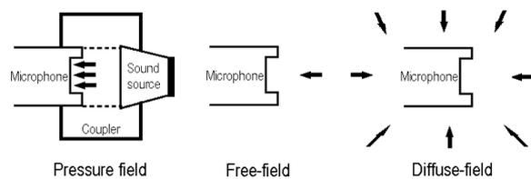
**Figure 1.** Sound fields for microphone calibration.
