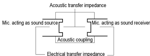
**Figure 2.** Procedure for primary calibration by reciprocity.
