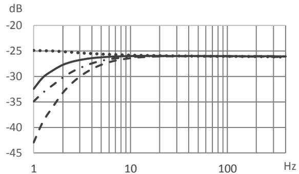
**Figure 5.** Measurements of microphone's and of microphone combined with preamplifier's cut-off. — for microphone (Brüel and Kjaer type 4145) with vent facing the sound field, - - for microphone combined with preamplifier (Brüel and Kjaer type 2673) also with vent facing it. · · · for the microphone with vent not facing the sound field and a · — · for the microphone combined with the preamplifier also with vent not facing it.
