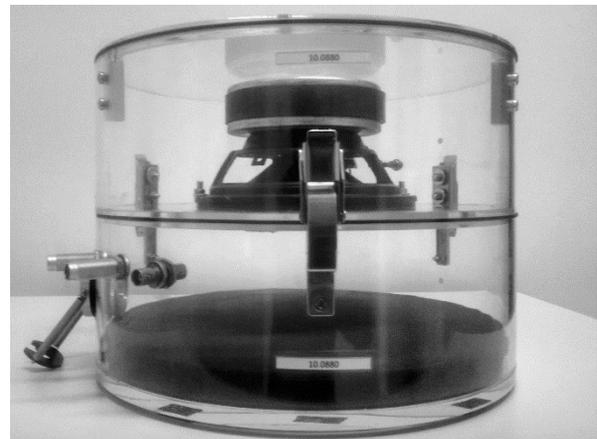
**Figure 6.** The sound pressure chamber used to calibrate microphones at low frequencies.
