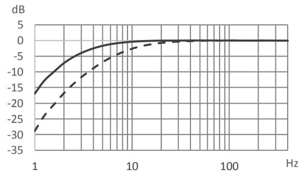
**Figure 3.** Microphone and preamplifier combined cut-off for different combinations. — for microphone 1 (Brüel and Kjaer type 4145) and preamplifier 1 (Brüel and Kjaer type 2673) and -- for microphone 2 (Brüel and Kjaer type 4191) and the same preamplifier 1.
