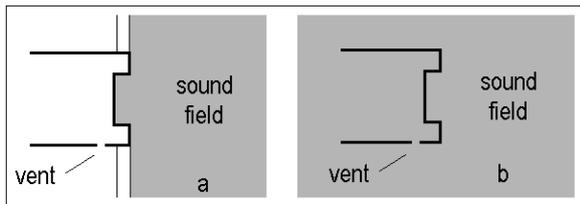
**Figure 1.** Measurement microphone with the equalization vent: (a) not facing the sound field and (b) facing it.
