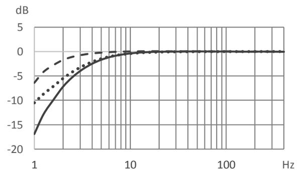
**Figure 4.** Individual frequency responses for microphone and preamplifier. — for microphone (Brüel and Kjaer type 4145) and preamplifier (Brüel and Kjaer type 2673) together, -- for the microphone and ··· for the preamplifier.
