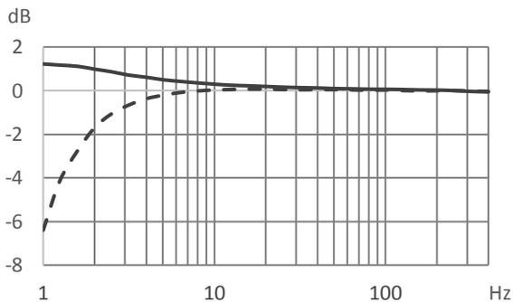
**Figure 2.** Frequency response of one-inch microphone (Brüel and Kjaer type 4145). — for microphone with vent not facing the sound field and -- for microphone with vent facing it.
