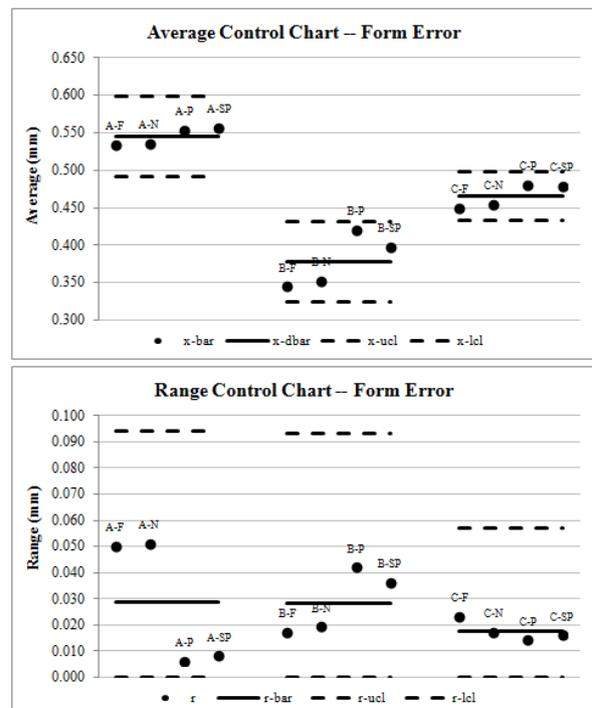
**Figure 2.** Control charts of the form errors of the datum planes exhibiting no out-of-control points.
