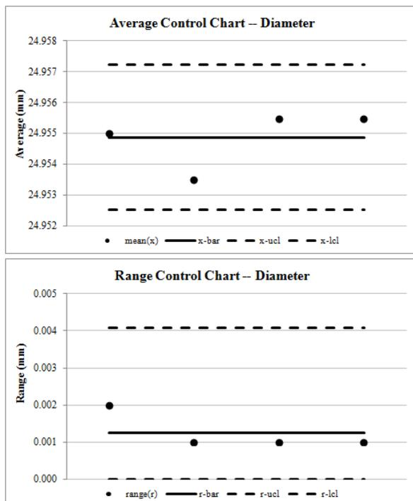
**Figure 3.** Average and range control chart of the hole diameter estimated with different presets.
