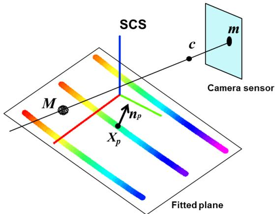
Figure 3. 3D point  $M$  defined at point cloud fitted plane.
