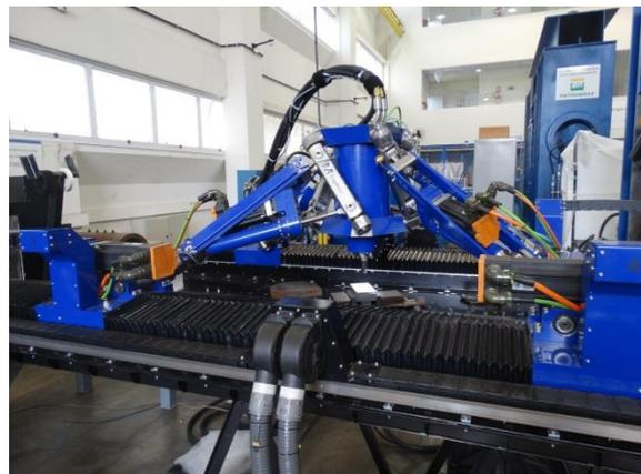
Figure 1. Closed chain robot with a friction stir welding head.
