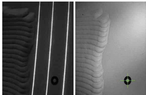
Figure 4. Laser image for point cloud calculation (left) and reference target image (already detected) for  $M$  calculation (right).
