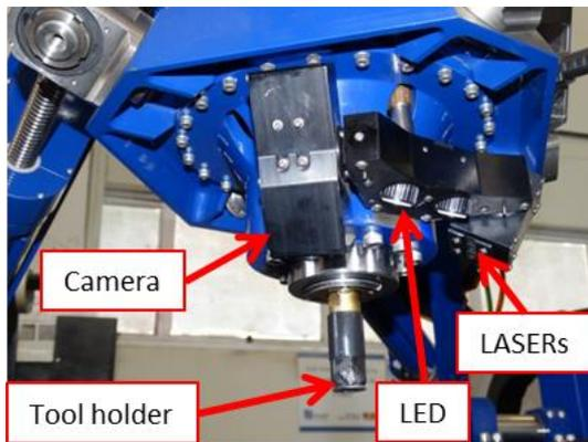
Figure 2. Sensor integrated with the robot.
