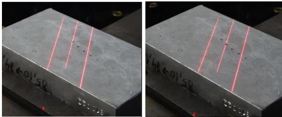
Figure 6. Central laser line already aligned with the first mark (left) and with the second mark (right).
