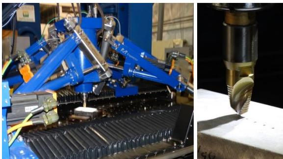
Figure 7. Friction stir welding head positioned for pin insertion process (left) and a detail of the tool aligned at first mark (right).
