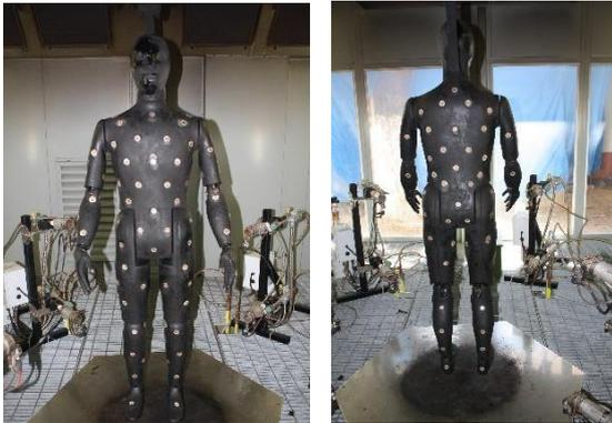
**Figure 1.** The instrumented manikin of SENAI-CETIQT (front view on left and back view on right).
